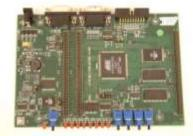
The microcontroller used in the demo is the Atmel EB63 Arm7 board, which runs at 25MHz. This board is loaded with the Microsoft Invisible Computing platform. Tasks include polling the gyro and managing the web services used to communicate with Robotics Studio. Because the board has no Ethernet port, the Ethernet packets generated by the network protocol are sent via a serial line to the PC and are then forwarded using a Virtual NIC driver.
