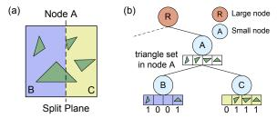
**Figure 3:** Storing triangle sets as bit masks of small root. Node A is split into node B and node C as shown in (a). Triangles B and C are subsets of their small root A's triangles. They are stored as bit masks as shown in (b).
