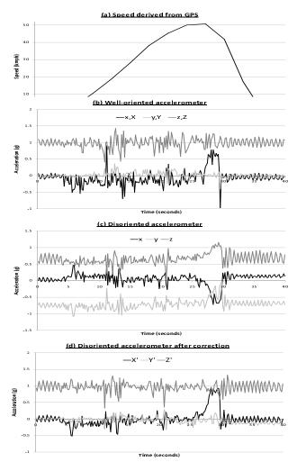
Figure 4: Estimating the orientation of a disoriented accelerometer based on sharp deceleration starting at around 27 seconds:  $\phi_{pre} = -88^{\circ}$ ,  $\theta_{tilt} = 49^{\circ}$ ,  $\psi_{post} = -135^{\circ}$
