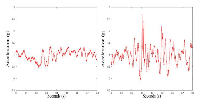
Figure 6:  $a_Z$  when traversing a bump at low Figure 7:  $a_Z$  when traversing a bump at high speed speed
