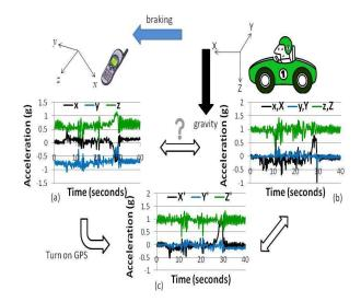
Figure 3: This figure illustrates the process of virtually reorienting a disoriented accelerometer. (a) shows the measurements made at a disoriented accelerometer, which unsurprisingly do not match with the measurements shown in (b), corresponding to a well-oriented accelerometer. However, after the disoriented accelerometer has been virtually reoriented, its corrected measurements shown in (c) match those in (b) quite well.
