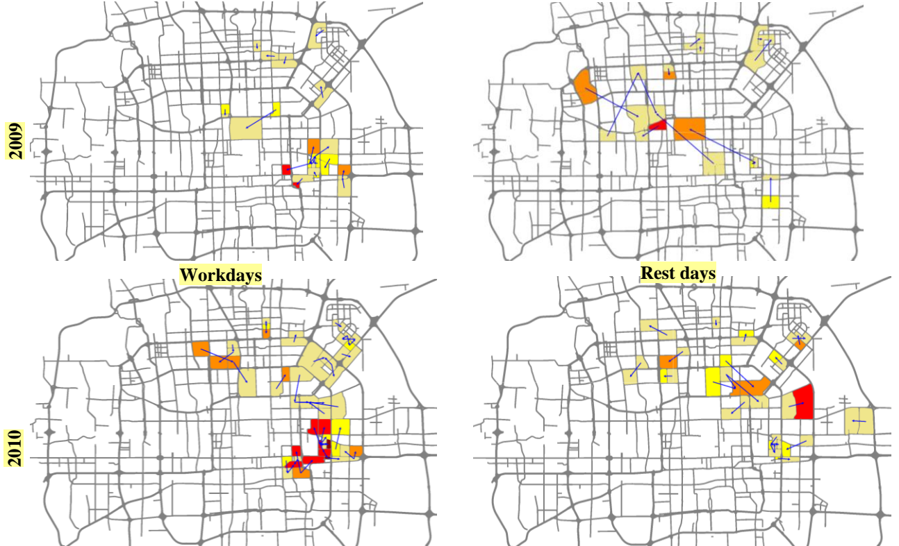
Figure 13. The flawed urban planning detected based on the taxi trajectories of 2009 and 2010 in the workdays and rest days: The color of a region denotes the frequency that a region has been detected as a flaw (the deeper means more frequent), and the arrows represent the direction of transition between two regions. The first row shows the results of 2009 and the second row stands for 2010. Figures in the left column pertain to workdays and the other column belongs to the rest days. The results are frequent sub-graph patterns with a support \geq 0.06 . Clearly, a hot region shown in Figure 12 might not be the region with frequent traffic problem, vice versa.
