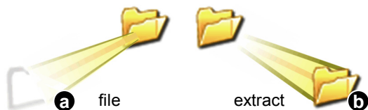
Figure 7: The tapered path indicates that (a) the folder at the bottom left was dropped into the other folder or (b) expanded from it.
