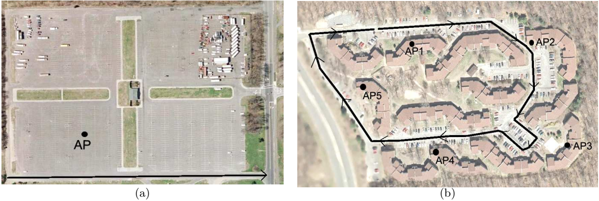
Figure 8: Two environments for the controlled experiments: (a) a large empty parking lot in the Stony Brook university campus, (b) a student apartment complex in the same campus. The black dots show the AP locations and the black arrow shows the driving route.
