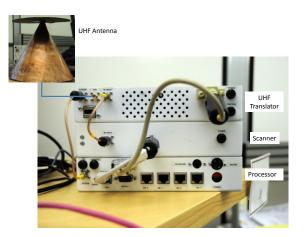
Figure 3: Photograph of the KNOWS hardware prototype.
