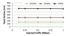
Figure 6: Accuracy of air time utilization measurement using SIFT. Error bars were within 2% of the mean.
