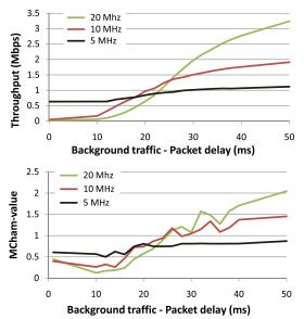
Figure 10: *MCham* value and resulting throughput of a 5, 10, and 20 MHz channel as a function of background traffic intensity. The *MCham* metric accurately predicts which channel achieves highest throughput.
