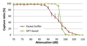
Figure 7: Discovery of APs with distance. SIFT is able to discover APs until as long as the Wi-Fi card can decode packets.
