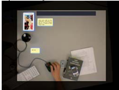
Figure 6. The WiM offers a real-time view of the desk to facilitate placement and interaction with virtual objects.
