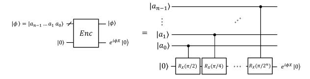
FIG. 7: Implementation of the phase encoding Enc of an n-bit string  $\phi = a_{n-1} \dots a_1 a_0$  using controlled rotations. The cost for each controlled rotation depends on the overall target error  $\epsilon$  and scales as  $O(\log 1/\epsilon)$  and is assumed to be the same for all rotations shown in the figure.
