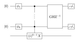
FIG. 3: Generalized PAR circuit with k inputs, where  $\mathrm{GHZ}^{-1}$  is the inverse GHZ measurement. Success is achieved if every measurement reads 0.
