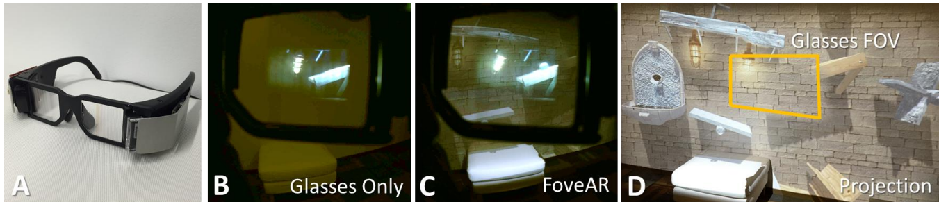
Figure 1. When using optically see-through display glasses (A), the viewer is presented with a limited field of view, impacting their sense of immersion and presence (B). FoveAR extends the glasses experience (C) by adding a view-dependent projection in the environment (D). Note: All first person images in this paper were photographed through the glasses. Due to the relative brightness of the glasses display and limited dynamic range of the camera, projected content appears subjectively dimmer than in reality.
