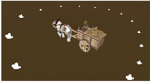
Figure 4: FLASHBACK caches dynamic objects by rendering a megaframe from all possible relative player positions and viewing angles, depicted here as camera icons. This repeats for all object animations and rotations.
