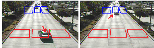
Figure 2: Step-by-step process of mapping traffic flow. Left: a vehicle entering the entry box. Right: a vehicle entering exit box.
