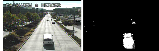
Figure 3: Background subtraction. Left: a vehicle entering the camera view. Right: binary mask indicating moving objects.
