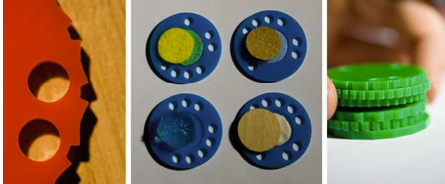
Fig. 4.1 Physical token design: ( left ) red task token with edge texture corresponding to the task owner; ( center ) blue document tokens with material attachments for identification; ( right ) green contact tokens with edge texture corresponding to other people in workgroup
