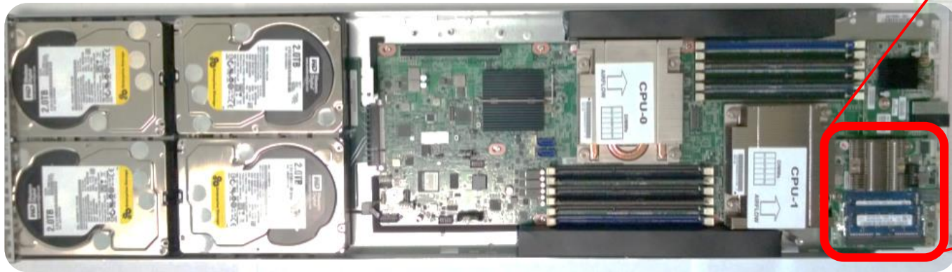
Data Center Server (1U, ½ width)
