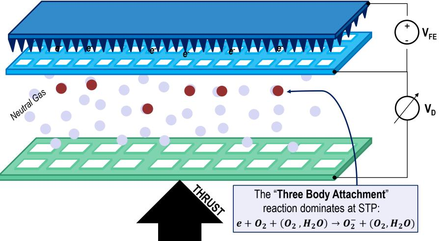
"Quadcoptor"-esque design, with individual thruster control from either field emission voltage or cathode-anode distance actuation.
