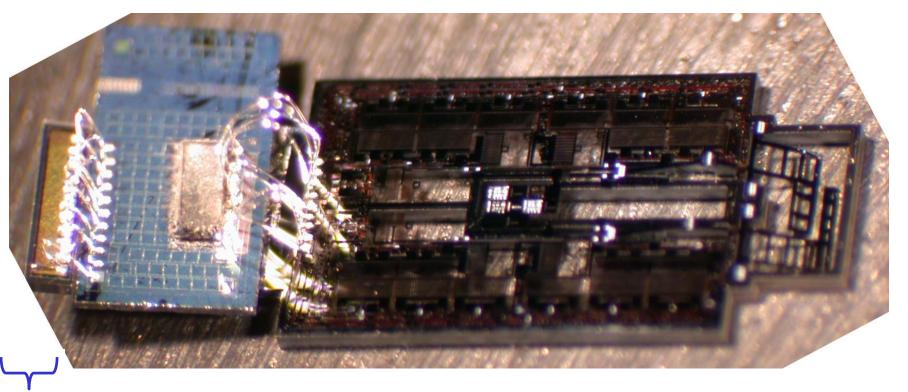
CMOS Sequencer Motors 8.6 mm
