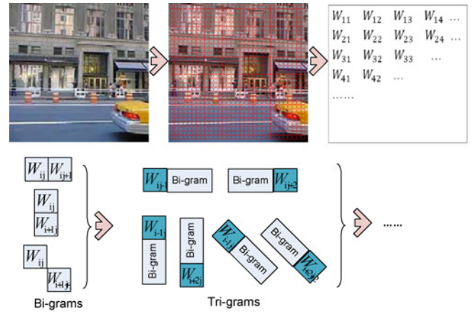
Fig. 5. Illustration of the visual N -grams extraction. The top middle image shows the extracted local features from the top left image, and the features are converted to visual words as at the top right image. The below figures illustrate the “visual N -grams” we define.
