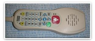
Figure 2: Remote control with large red call button
