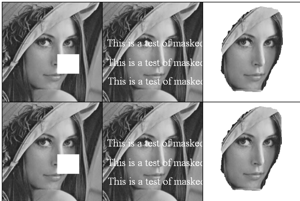
Figure 4. 256 \times 256 masked image coding result, for PSNR = 40 dB for unmasked pixels. Top: PWC/POCS; bottom: proposed masked wavelet codec. Note the absence of artifacts near the mask boundaries. The proposed wavelet coder is an order of magnitude faster than PWC/POCS.
