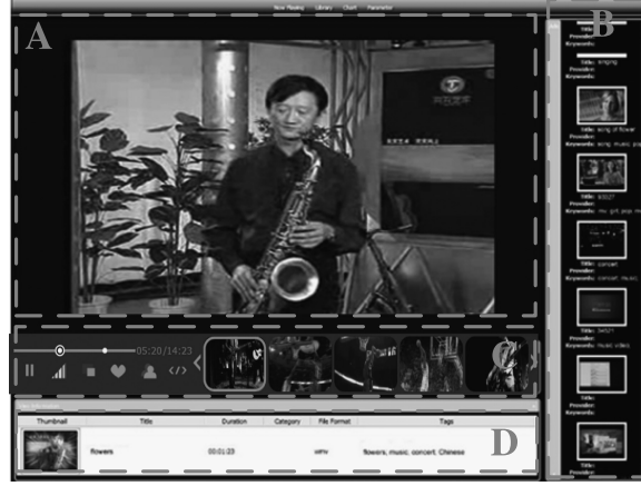
Fig. 4. User interface of our video recommendation system. A—online video; B—recommended video list; C—shot list, the highlighted shot indicates current playing content; D—related textual description of this online video.
