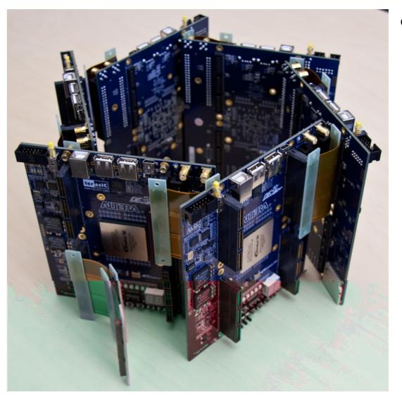
• FPGAs allow us to run test programs at a decent speed, without having to do a full, expensive and inflexible silicon implementation.
