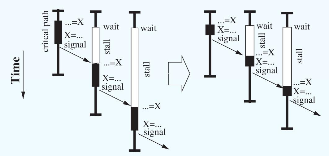
A compiler can schedule instructions to reduce the *critical forwarding path*, therefore increasing parallel overlap and improving performance by placing **wait** instructions as late as possible and **signal** instructions as early as possible in the code.
