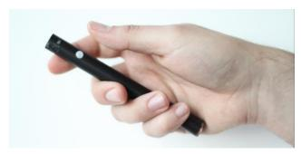
Figure 14: Custom IR laser pointer.
