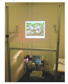
Figure 2 TouchLight prototype. Note two cameras clearly visible behind transparent projection display.
