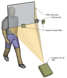
Figure 1 TouchLight physical configuration: DNP HoloScreen with two IR cameras and IR illuminant behind screen.
