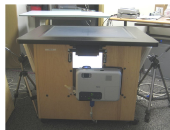
Figure 5: Area antennas can be unobtrusively added to front- and rear-projected systems. RFID tags are detected in the overlapping volume of the transmission (TX) and reception antenna (RX).
