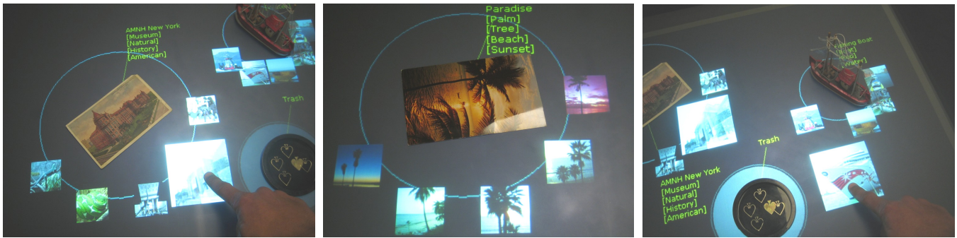
Figure 8: Our tangible image explorer enables interaction with unobtrusively tagged physical objects on interactive surfaces.
