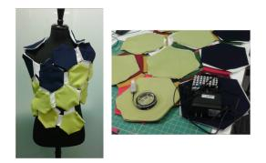
Figure 2. Cotton fabric scarf includes detachable hexagonshaped modules enclosing hardware such as battery-powered vibration modules and heat coil pads
