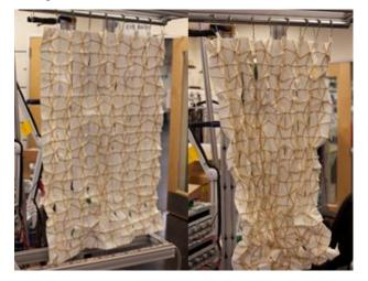
Figure 5. Textile Mirror Prototype (left) relaxed (right) stressed
