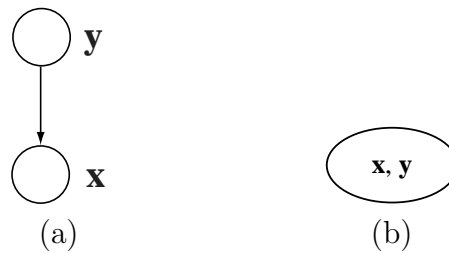
Figure 5-9: A factor analyzer as a hybrid Bayesian network and its (trivial) clique tree.
