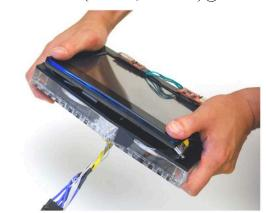
Figure 1: GyroTab provides reactive torque feedback. Two masses (under the display) spinning in opposite directions are controlled to produce varying levels of feedback that oppose the user's movement.
