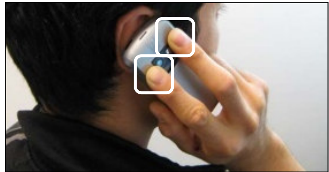
Figure 9. This typical phone holding posture places index and middle fingers on the back of the device.
