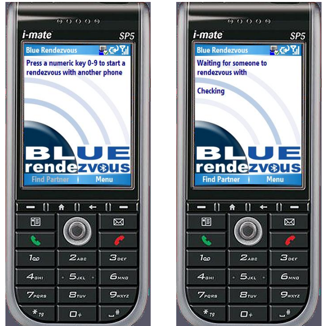
Fig. 1. Left: BlueRendezvous welcome screen. Users connect by pressing the same numeric key at about the same time. Right: After simultaneous key presses, the devices attempt to discover one another.
