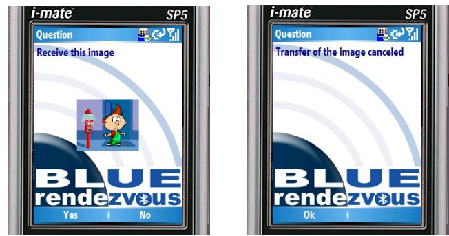
Fig. 8. Left: A user sees a thumbnail preview of the image that another user is transmitting, and can choose whether or not to accept it (Yes/No). Right: Hitting NO allows the receiving user to veto the transfer from the other device.
