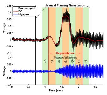
Figure 3: Down-sampled data (solid black), DC waveform (dashed red), and high-pass filtered data (solid blue) for a rotate gesture (5). The manual framing timestamps are shown (black), as well as the segmentation timestamps determined by the segmentation algorithm (red). Each of the windows used for feature extraction are also shaded.
