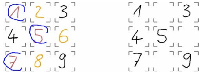
Figure 6. Task screen: The user has just circled (1,5,7) with ink (left grid). The user then switches to gesture mode, selects the numbers highlighted in orange (2,6,8), and uses the Move command to drag them to the empty slots (at right).
