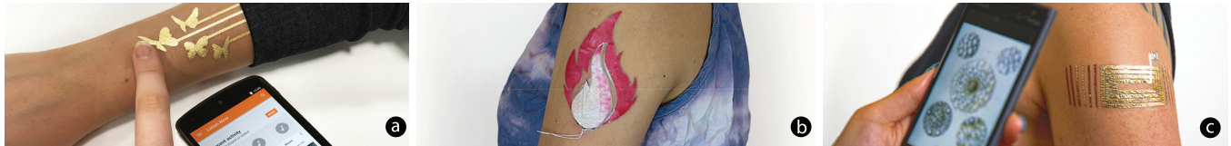
Figure 1: DuoSkin is a rapid prototyping and fabrication process using the skin-friendly material gold leaf to create wearable on-skin user interfaces, such as (a) sensing touch input, (b) displaying the user’s mood using a thermochromic tattoo, and (c) communicating and sharing data with other devices through NFC—all while maintaining body decoration aesthetics.
