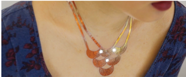
Figure 9: Aesthetic customization: LED skin necklace. The color is customized with variegated leaf, and the traces are decorative while serving as functional circuitry
