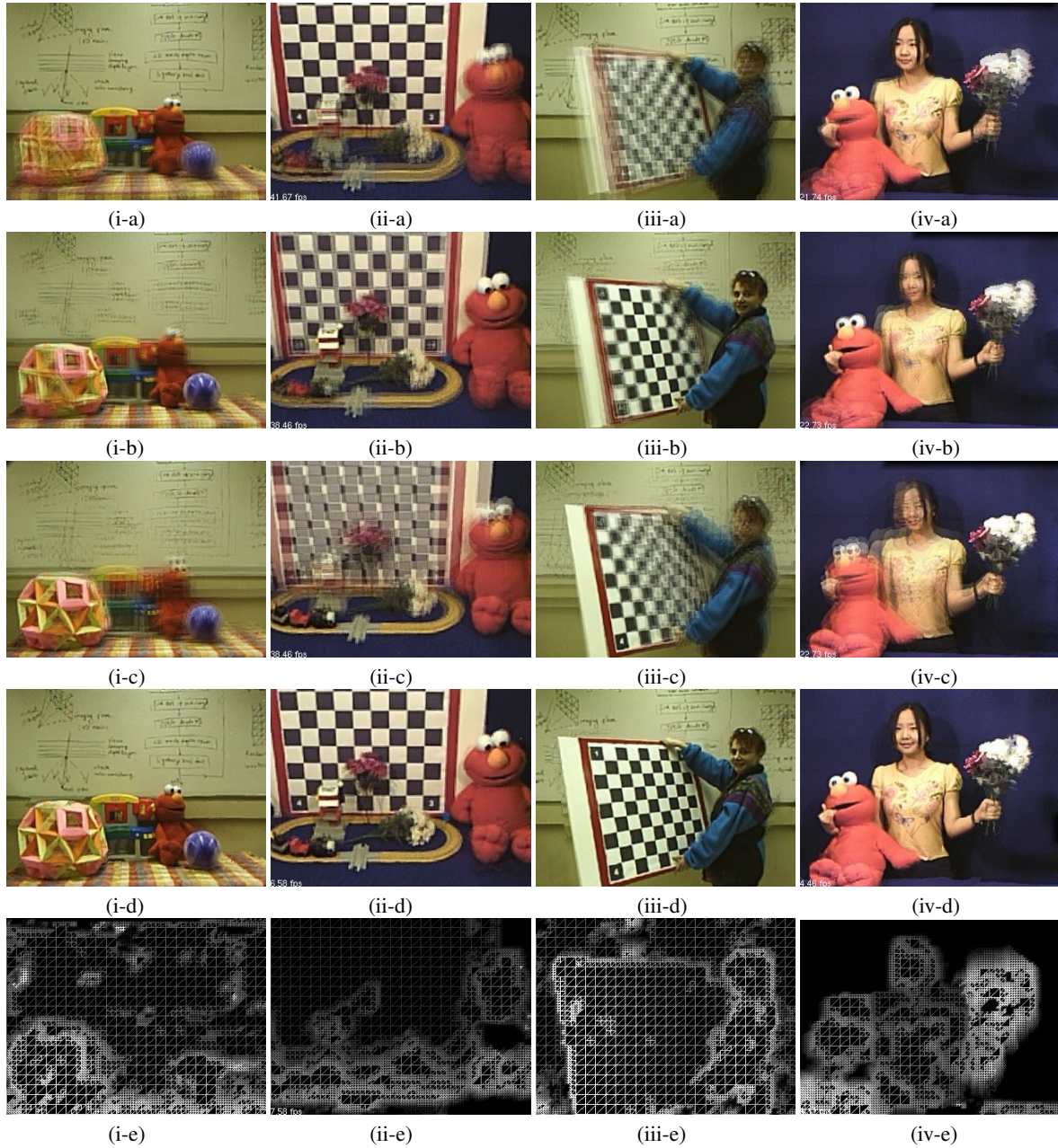
Figure 9: Scenes captured and rendered with our camera array (no camera motion). (i) Toys scene. (ii) Train scene. (iii) Girl and checkerboard scene. (iv) girl and flowers scene. (a) Rendering with a constant depth at the background. (b) Rendering with a constant depth at the middle object. (c) Rendering with a constant depth at the closest object. (d) Rendering with the proposed method. (e) Multi-resolution 2D mesh with depth reconstructed on-the-fly. Brighter intensity means smaller depth.
