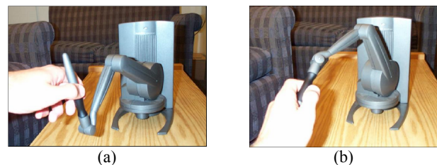
FIGURE 2: The grip used by the player significantly affects the structural impact that gameplay has on the haptic device. (a) correct grip, (b) incorrect grip, shown at this device’s singularity
