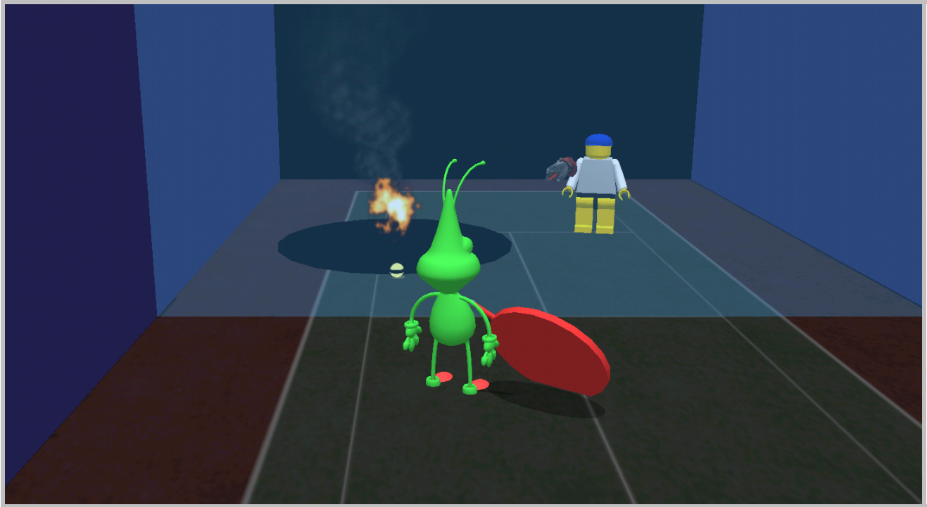
FIGURE 1: A screen shot captured from Haptic Battle Pong. Each avatar represents the center of a player’s haptic workspace; players control tools in six degrees of freedom within that workspace.
