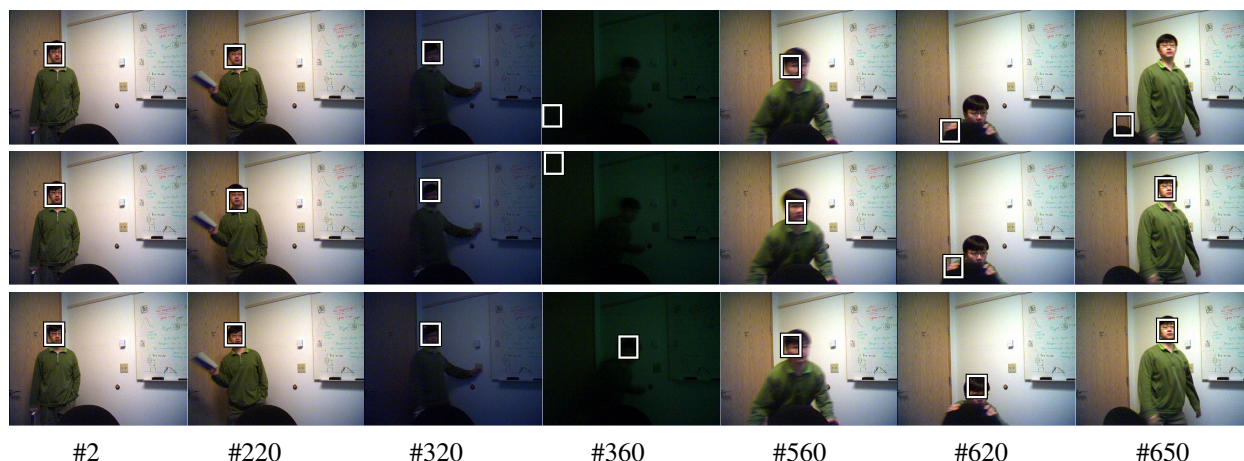
Figure 6. Office sequence. The frames 2, 220, 320, 360, 560, 620 and 650 are shown. The top row is the result of a MS tracker; the middle row is the result of a MSBM tracker; the bottom row is the PCI tracker with appearance modeling.
