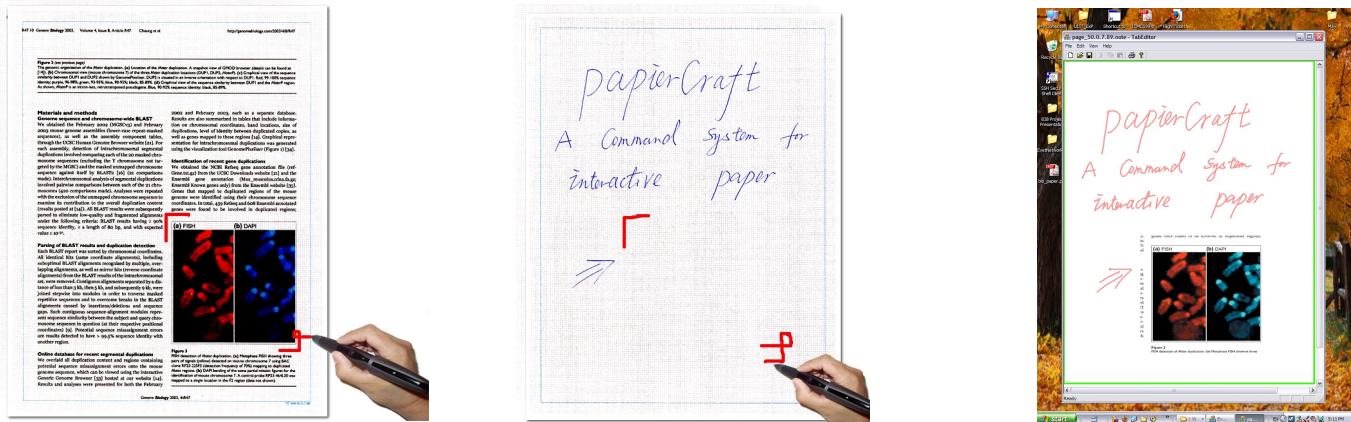
Figure 1 A copy/paste interaction in PapierCraft: an image is copied from a printout (left), then pasted to a note (center). The result is shown on our PapierCraft viewer after pen synchronization (right). Marks were highlighted for clarity. Page from Open Access document http://genomebiology.com/2003/4/8/R47 © 2003 Cheung et al. Used with permission.
