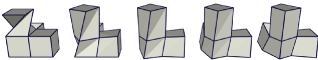
Figure 5: PQ perturbation without a closeness term applied to a highly un-planar mesh consisting of only a few quads.
