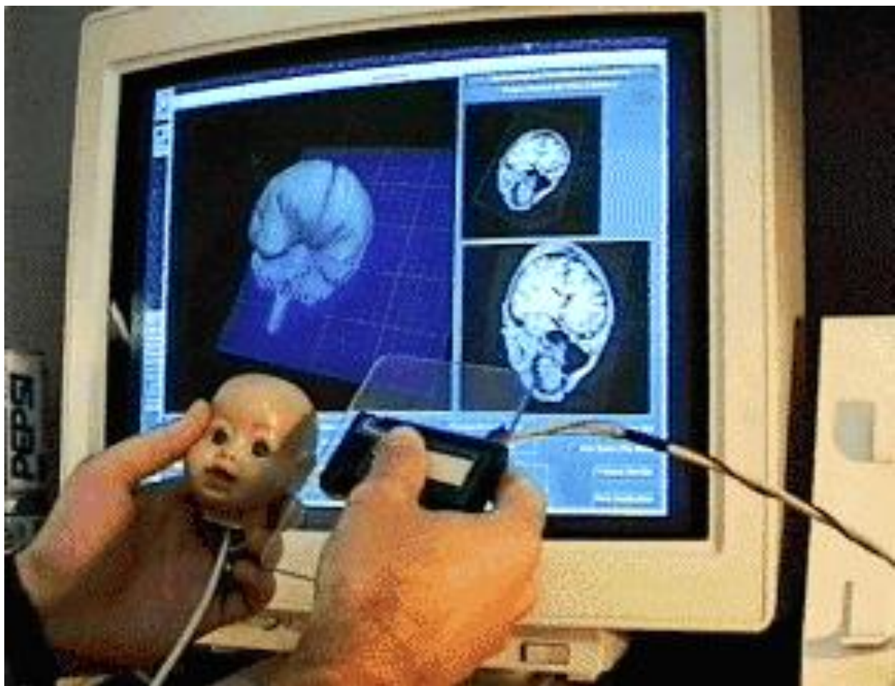
Figure 1: User selecting a cross-sectioning plane using the two-handed props interface for neurosurgical visualization.
