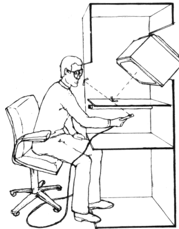
Figure 2.8 Schmandt's stereoscopic workspace [142].
