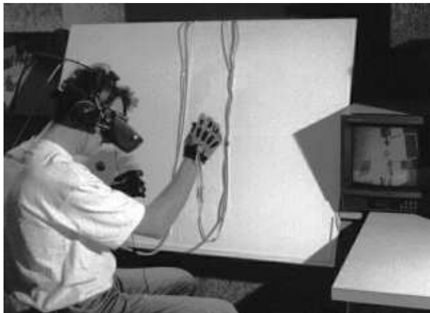
Figure 2.5 Polyshop employs two-handed interaction with chord gloves [1].
