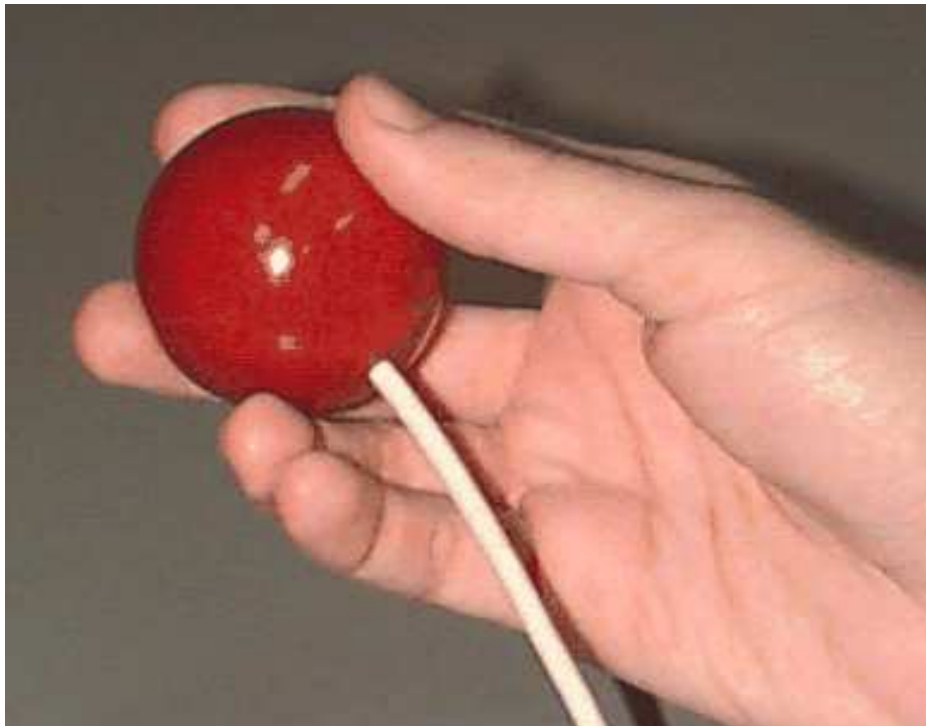
Figure 6.2 The 3D Ball input device.
