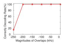
Figure 8. Reliability vs magnitudes of subcarrier overlap
