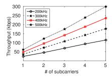
Figure 9. Throughput vs # of subcarriers in SNOW
