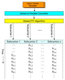
Figure 2. Steps of packet decoding
