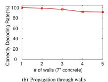
Figure 6. Link level experiment over obstacles (indoor)
