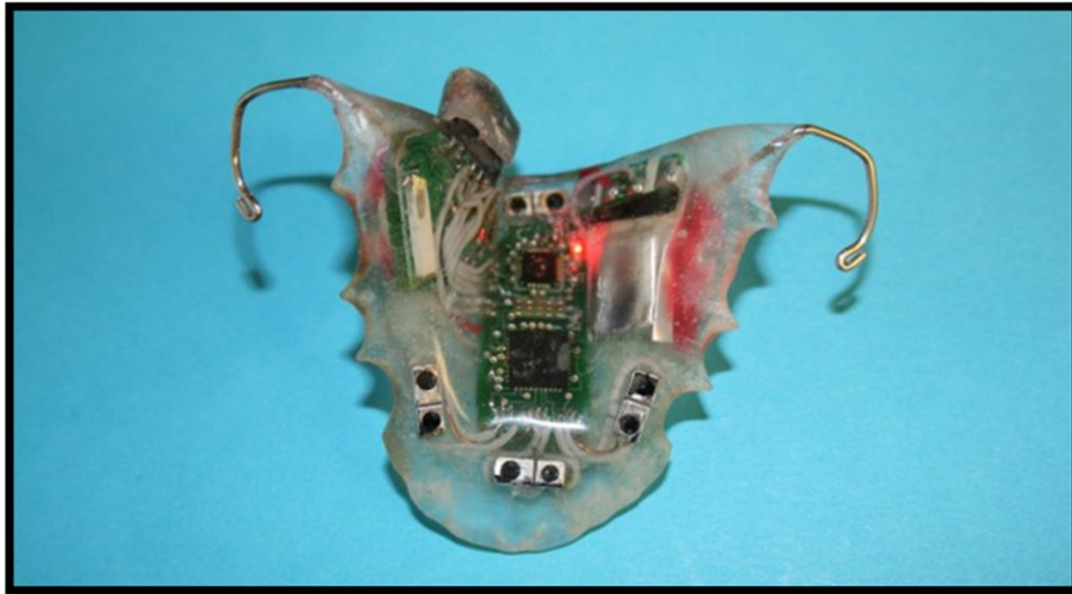
Figure 7-2: Our infrared based wireless tongue computer interface embedded in an acrylic retainer.
