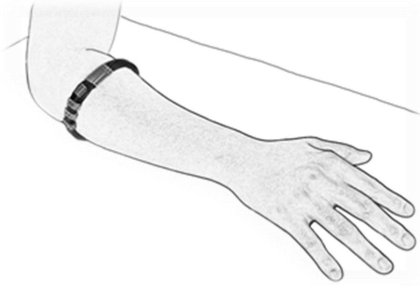
Figure 3-4: Artist rendering of a forearm band with EMG sensors that could be used for muscle-computer interfaces.
