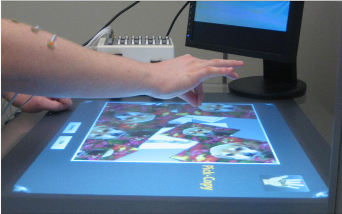
Figure 6-8: Performing the finger-dependent pick and throw interaction: A user picks up a virtual object by pinching it on the surface and lifting his hand away from the surface. Releasing the pinch returns the object to the current canvas.
