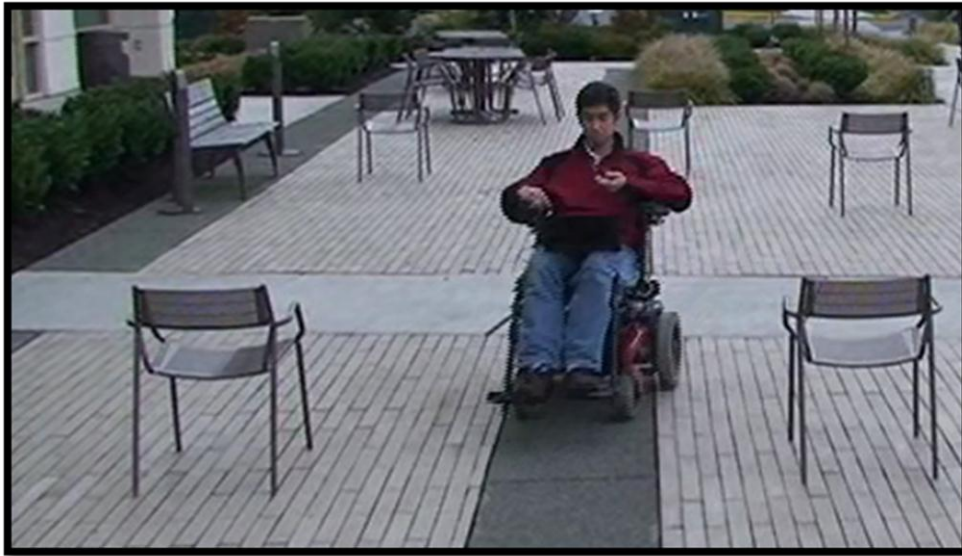
Figure 7-3: A person using our wireless tongue input platform to drive a motorized chair through an obstacle course.
