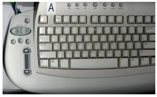
*Fig. 1.* Prototype A of the scrolling strip on the left pod of the Microsoft Internet Keyboard. (N.B: The shape of the strip differed slightly in Rounds 1 and 2.)
