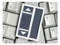
*Fig. 13.* Scrolling strip with absolute function in the "sawtooth" area on the right side of the strip.
