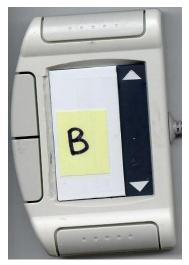
*Fig. 4. Prototype B, a scrolling strip without arrow separations.*
