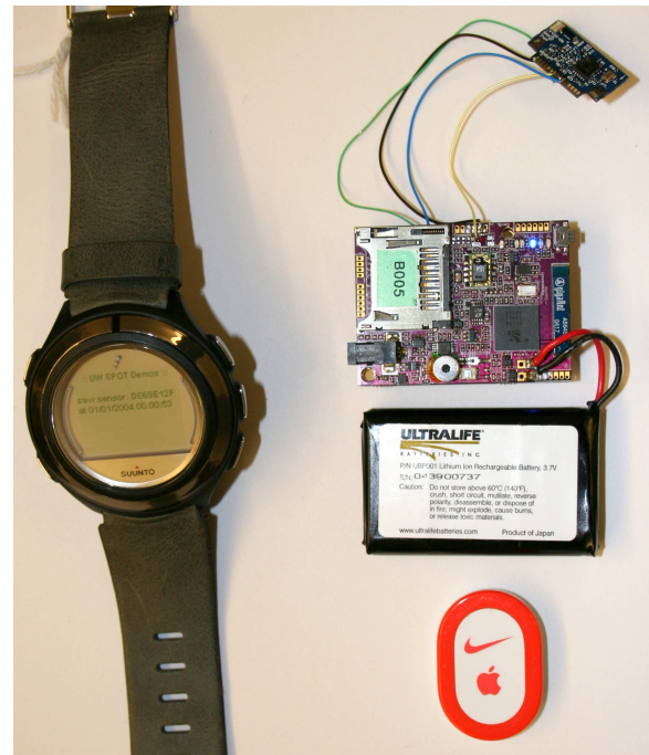
Figure 9: A Microsoft SPOT Watch receiving Nike+iPod sensor IDs from an iMote2 over wireless bluetooth.
