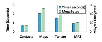
Figure 4. Performance overhead upon device lock.
