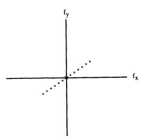
Fig. 9. Fourier transform of grating.
