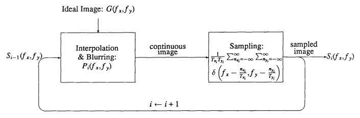
Fig. 13. Block diagram illustrating multiple stage reconstruction and sampling.
