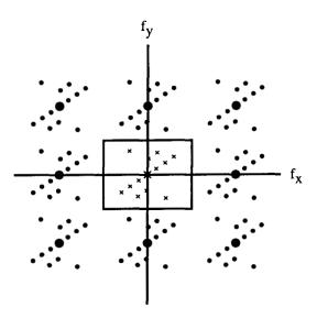
Fig. 11. Spectral orders after second stage sampling with no additional aliasing because of high frequency sampling.
