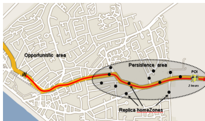
Figure 1: Black dots represent homeZones where messages should be stored to inform approaching vehicles about the road works (POI).
