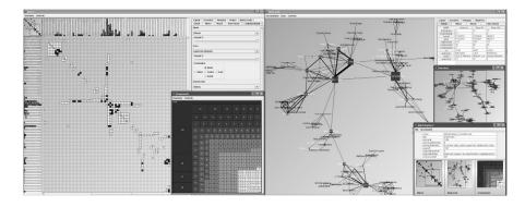
Figure 11. A screenshot of MatrixExplorer. This system combines matrices (left large window) and node-link diagrams (right large window). The smaller window on the left shows a treemap view of the macrostructure of the network (connected components). The windows in the lower right corner show miniature bird's eye views of the visualizations. Queries and textual data are shown in top windows.
