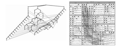
Figure 5. A network represented as tree plus additional links on the left. A network represented as a Treemap plus additional links on the right.
