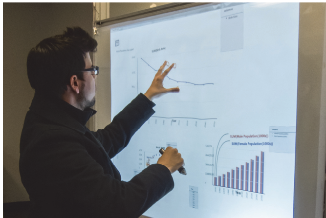
Fig. 1. A pen-and-touch whiteboard: a back-projected vertical surface that used an infrared Laser Light Plane (LLP) [41] to recognize touch, and an eBeam [25] device to provide pen functionality.
