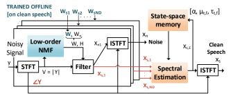
Fig. 3: Block diagram of the proposed NMFSE approach.
