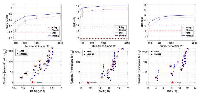
Fig. 7: Top: NMFSE improves NMF PESQ, SNR and SDR by up to 0.24, 2.76 dB and 4.37 dB, respectively. Bottom: runtimes with different values of  $N_D$ ; points corresponding to the upper figures ( $N_D$ =20) are highlighted with big markers.
